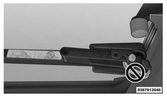
Improper Clamp Position
