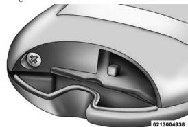
**Remove Screw From Transmitter Case**
