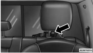
Tether Strap Through Outboard Tether Strap Loop
