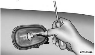
Removing Bulb Socket From Clearance Lamp
