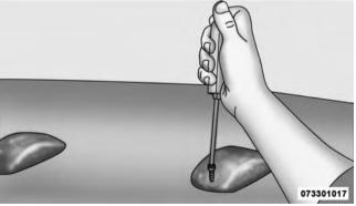
Removing Rear Screw From Clearance Lamp
