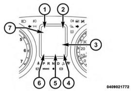
The EVIC displays are located in the center portion of the cluster and consists of seven sections:
