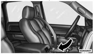
Inserting Latch Plate Into Buckle
