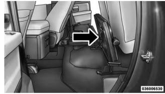
Load Floor Securing Straps/Quad Cab®
