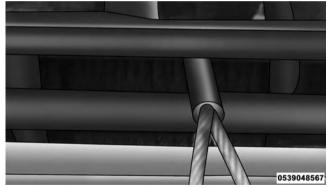
Wire Neatly Wound Around The Spooling Drum
