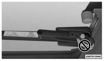
Improper Clamp Wire Released Position
