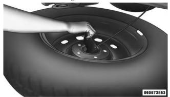
Reinstalling The Retainer
