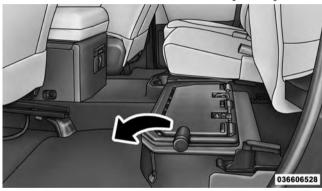
**Unfolding The Load Floor**
