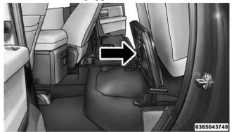
Load Floor Securing Straps/Crew Cab®
